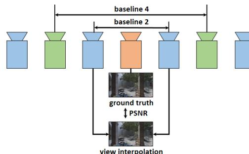
Figure 1: The camera setup of the datasets. The cameras are placed on a line, equally spread. We skip a number of cameras to simulate a larger baseline. The middle camera is always the ground truth camera, and is never used for view synthesis. This ground truth image is compared with the synthesized image using the PSNR metric.
