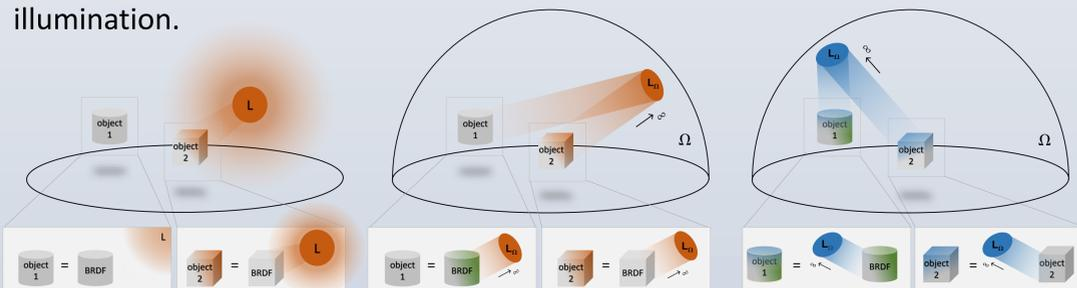
(left) A scene with 2 objects and a red local light source L. (middle) Current techniques model local lighting effects with distant light sources at infinity. This causes erroneous correction colors (shown here as green) in the BRDF. (right) Relighting reveals the wrongly estimated materials.
